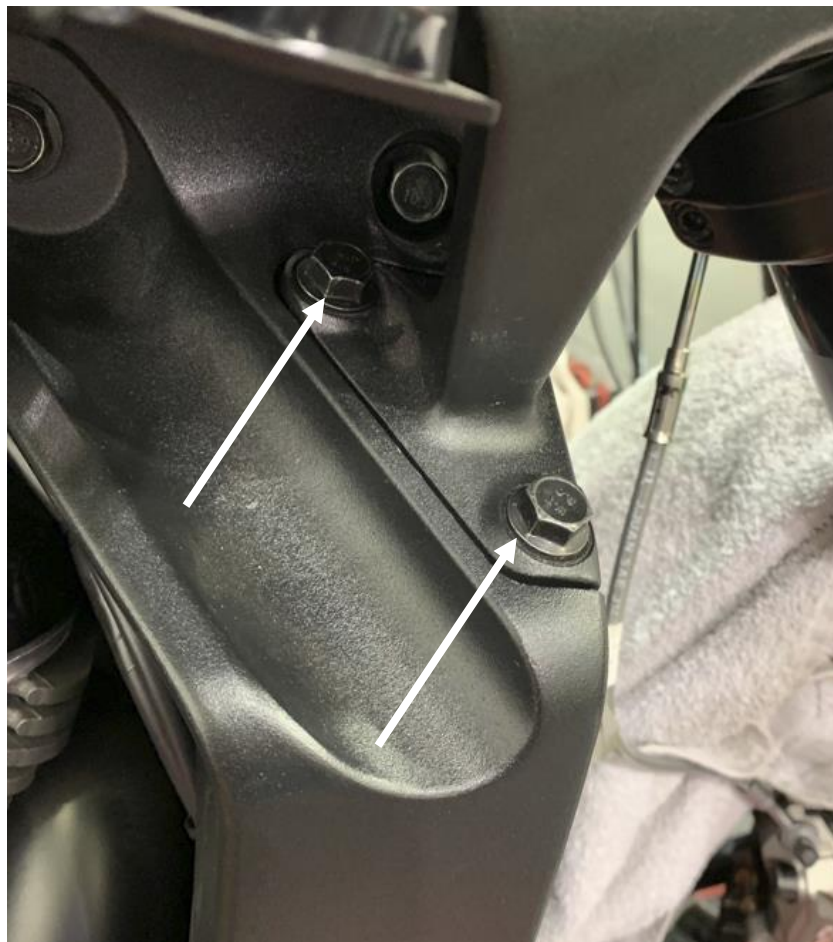
Figure 12: Remove the inner fairing frame fasteners (right side shown, left side similar).
