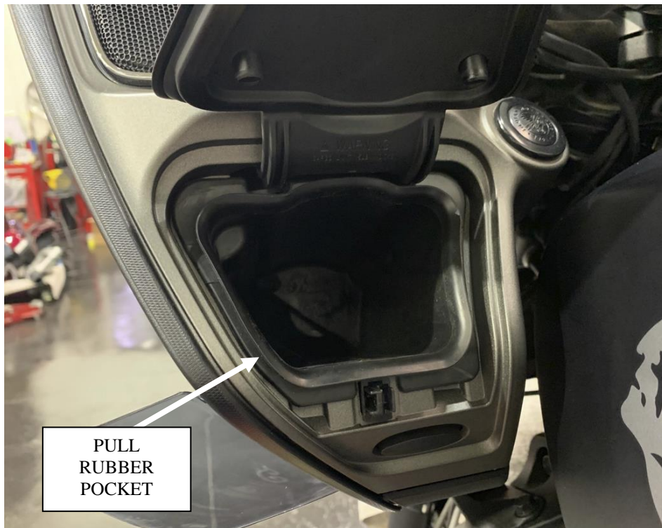
Figure 4: Remove the rubber pocket liners (left side shown, right side similar).
