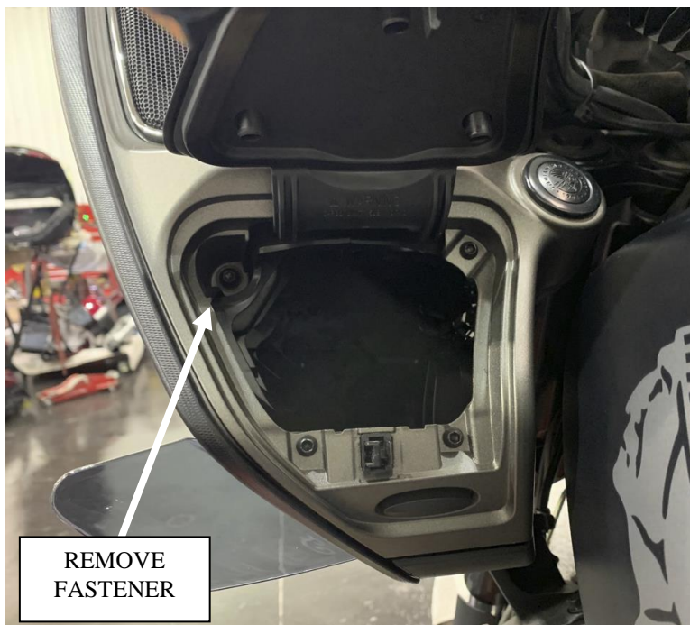
Figure 5: Remove torx fastener from upper outside corner (left side shown, right side similar).
